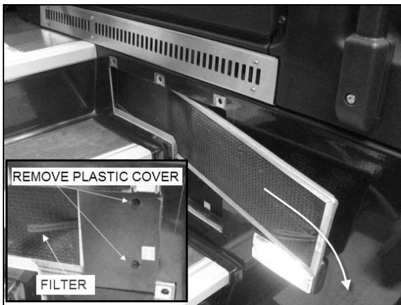
REMOVING DRIVER'S SECTION AIR FILTER
