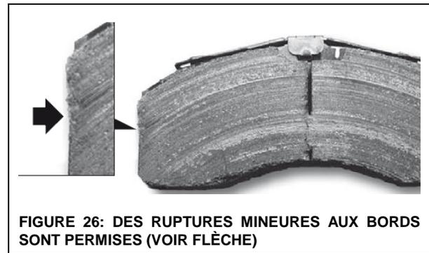
FIGURE 26: DES RUPTURES MINEURES AUX BORDS SONT PERMISES (VOIR FLÈCHE)
