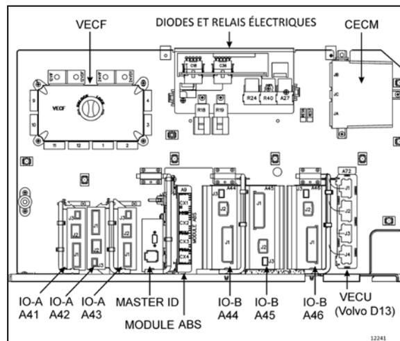
FIGURE 32: EMBLACEMENT D'ECU ABS
