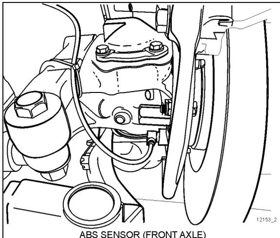
FIGURE 33: EMBLACEMENT DE CAPTEUR ABS
