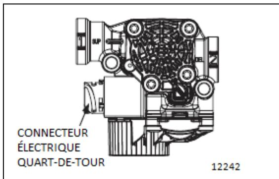
FIGURE 35: VALVE MODULATRICE DE PRESSION BENDIX M-40QR
