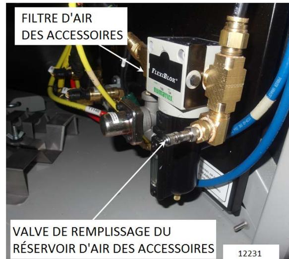
FIGURE 3: FILTRE DU COMPARTIMENT DE SERVICE AVANT 12231
