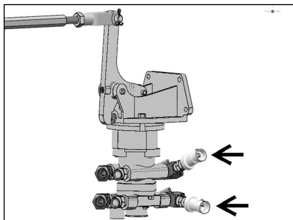
FIGURE 15: MANOCONTACT DE FEUX D'ARRÊT 12139
