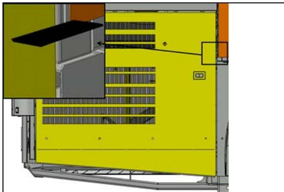
FIGURE 118: UTILISER UNE RÈGLE POUR VÉRIFIER SI LES SURFACES SONT AU MÊME NIVEAU
