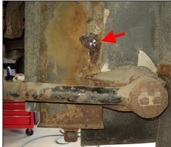
FIGURE 6: ZONE NETTOYÉE SUR LE CHÂSSIS
