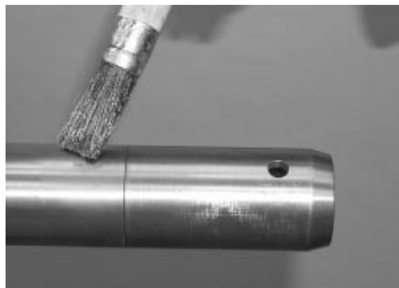
FIGURE 19: APPLY GLEITMO 805 GREASE
