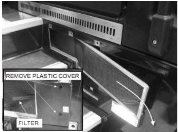
FIGURE 18: REMOVING DRIVER'S SECTION AIR FILTERS
