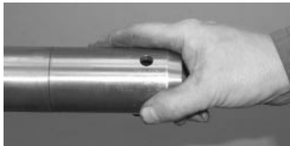
FIGURE 18: INSERTION TOOL PREVOST P/N 491115
