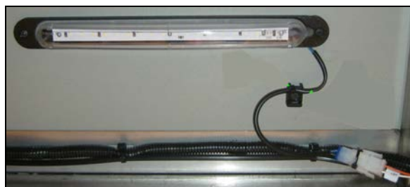
FIGURE 91: BAGGAGE COMPARTMENT LIGHTS LED SEALED UNIT
