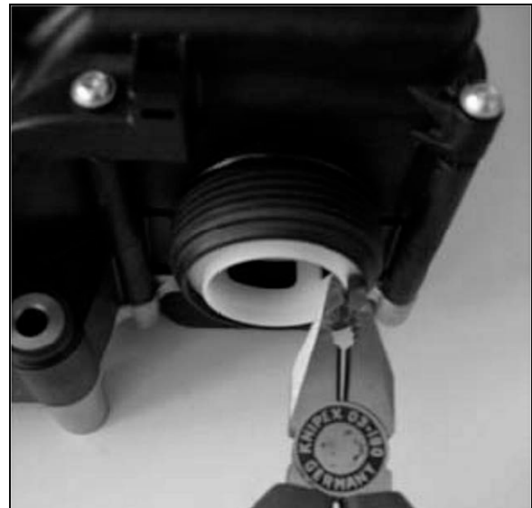
FIGURE 12 : PUMP ASSEMBLY FILTER ELEMENT
