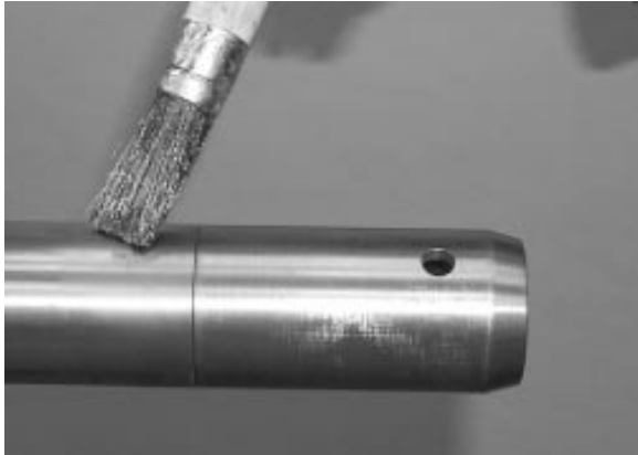
FIGURE 10: APPLY GLEITMO 805 GREASE
