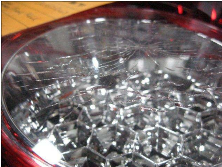
FIGURE 3: Cracking of the outer surface of the taillight due to the use of engine degreaser
