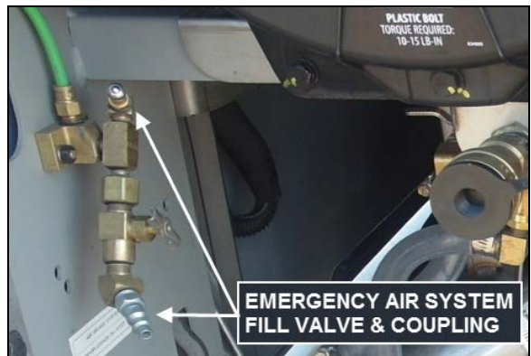
EMERGENCY AIR SYSTEM FILL VALVE AND COUPLING
