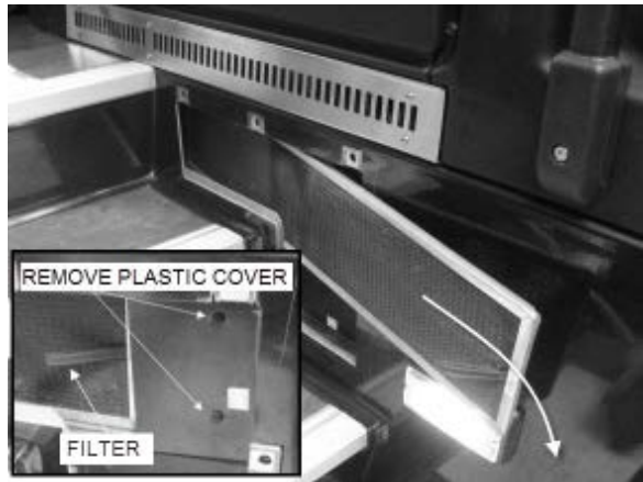
FIGURE 18: REMOVING DRIVER'S SECTION AIR FILTERS
