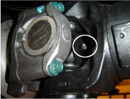
FIGURE 5: EMBOUT DE GRAISSAGE ZERK
