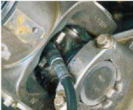
FIGURE 6: EMBOUT DE GRAISSAGE ZERK
