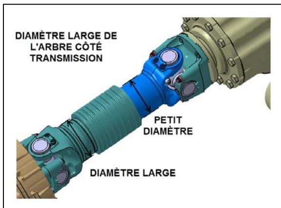
FIGURE 13: ORIENTATION CORRECTE DE L'ARBRE DE TRANSMISSION
