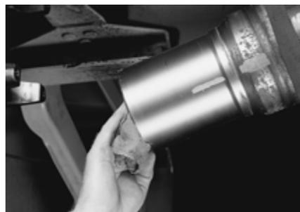
FIGURE 23: NETTOYER LA GRAISSE DU MANCHON CANNÉ
