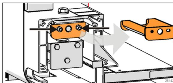
FIGURE 10: ENLÈVEMENT DE LA BUTÉE D'EXTENSION
