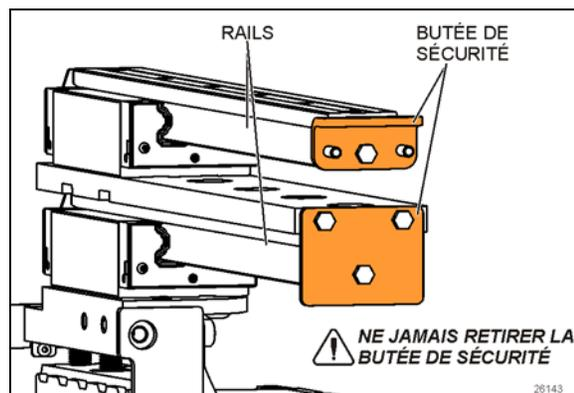
FIGURE 68: BUTÉES DE SÉCURITÉ SUR LES RAILS
