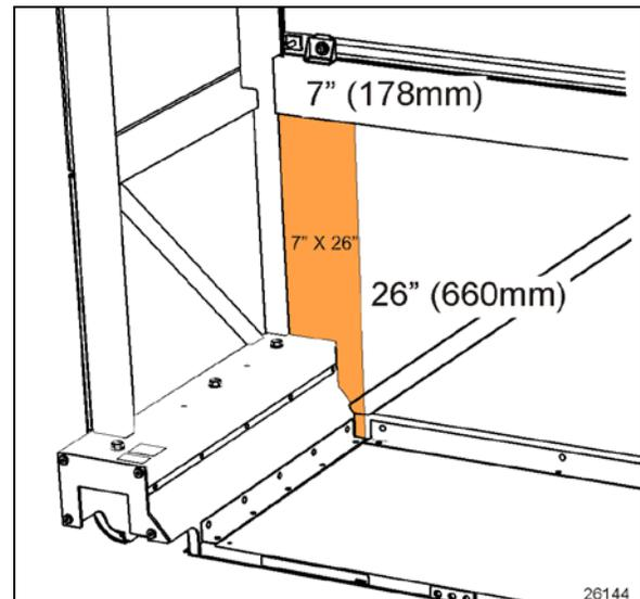
FIGURE 71: ZONE D'INTERDICTION DE PERÇAGE (AVANT ET ARRIÈRE)
