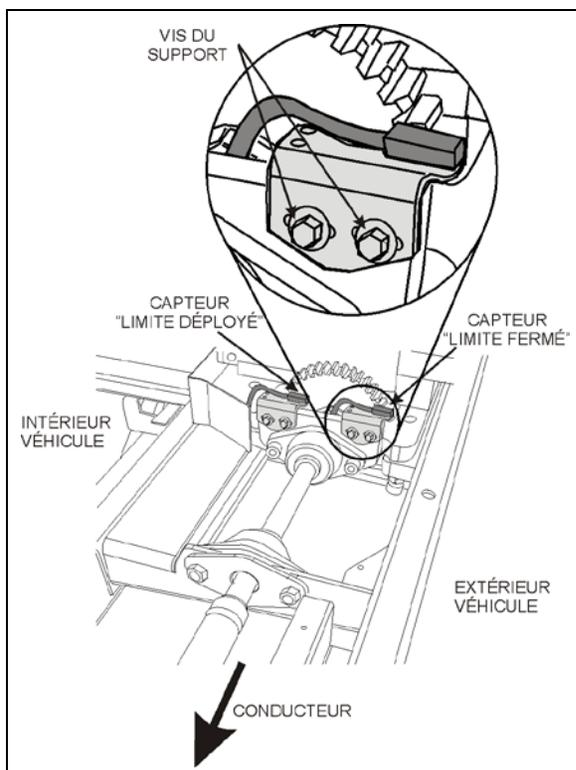
FIGURE 39: CAPTEURS D'EXTENSION 26073
