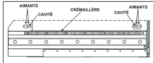
FIGURE 40: AIMANTS SUR LE SOUBASSEMENT D'EXTENSION 26097
