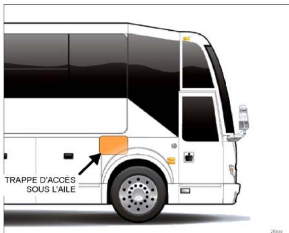
FIGURE 63: TRAPPE D'ACCÈS POUR LES VIS D'AJUSTEMENT POUR L'INCLINAISON ET MISE À NIVEAU
