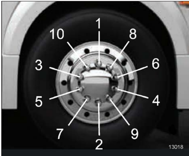
TIGHTENING SEQUENCE
