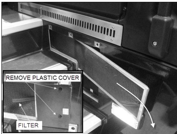
REMOVING DRIVER'S SECTION AIR FILTER
