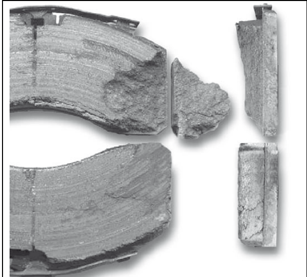
FIGURE 23: MAJOR BREAKOUTS ON THE SURFACE OF THE BRAKE PAD ARE NOT PERMITTED
