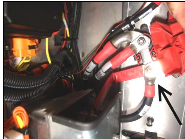
Figure 3: Bussman Junction Block - H3 Series.
