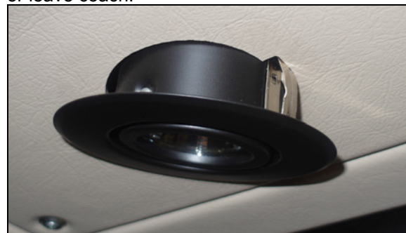
FIGURE 101: DRIVER'S AREA CEILING LIGHT
