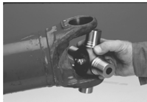
FIGURE 30: POSITION THE JOURNAL CROSS INTO THE YOKE CROSS HOLES WITH THE GREASE ZERK FITTING INWARD TOWARD TUBING
