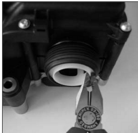
FIGURE 13 : PUMP ASSEMBLY FILTER ELEMENT
