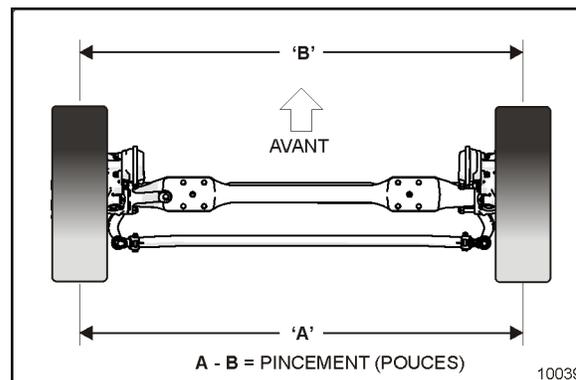
FIGURE 6: MESURE DE PINCEMENT
