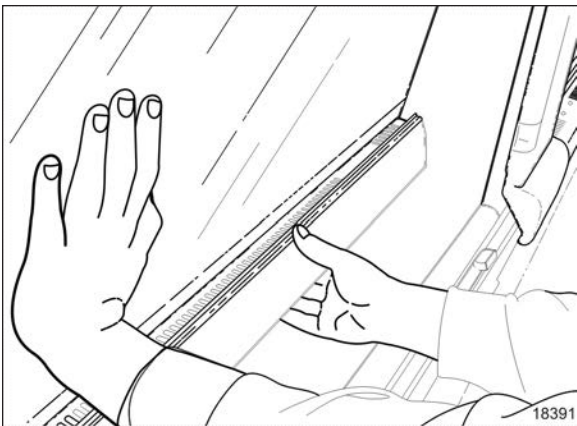
EMERGENCY WINDOW OPENING
