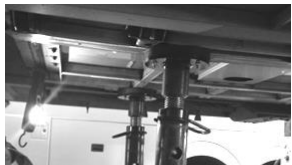
FIGURE 21: JACK STANDS UNDER THE FUEL TANK CRADLE
