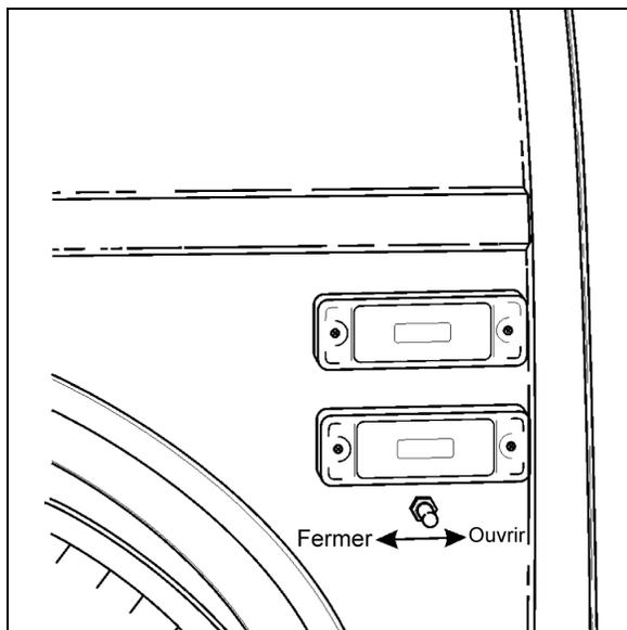
FIGURE 24: INTERRUPTEUR DE COMMANDE DE LA PORTE D'ENTRÉE 18599
