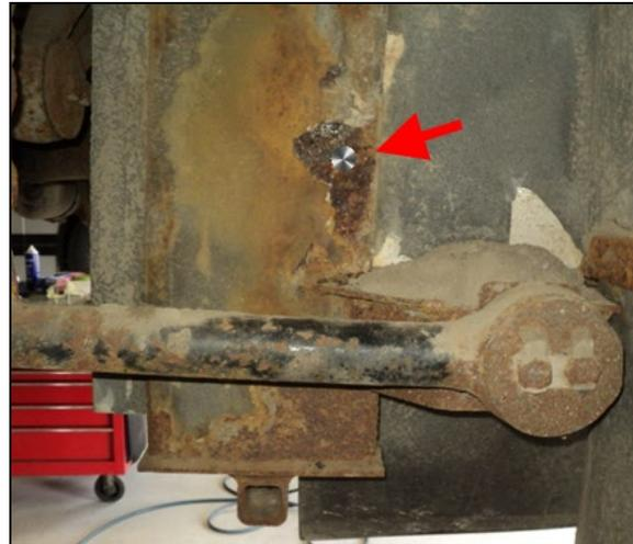
FIGURE 6: ZONE NETTOYÉE SUR LE CHÂSSIS
