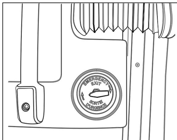
FIGURE 25 : SOUPAPE D'OUVERTURE D'URGENCE INTÉRIEURE 18330
