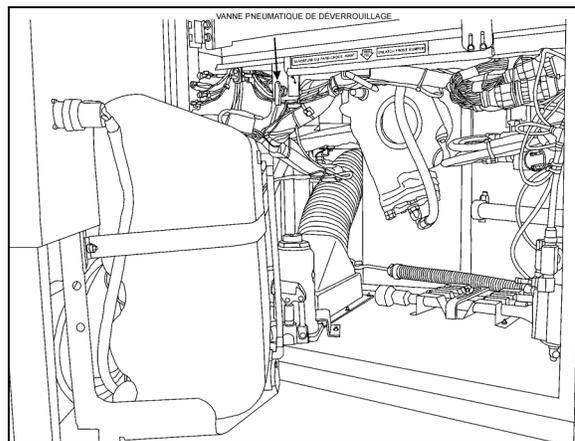
FIGURE 26: SOUPAPE D'OUVERTURE D'URGENCE EXTÉRIEURE 12209
