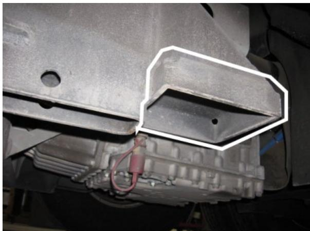
**FIGURE 15: SUPPORT DE LEVAGE AU CHÂSSIS
