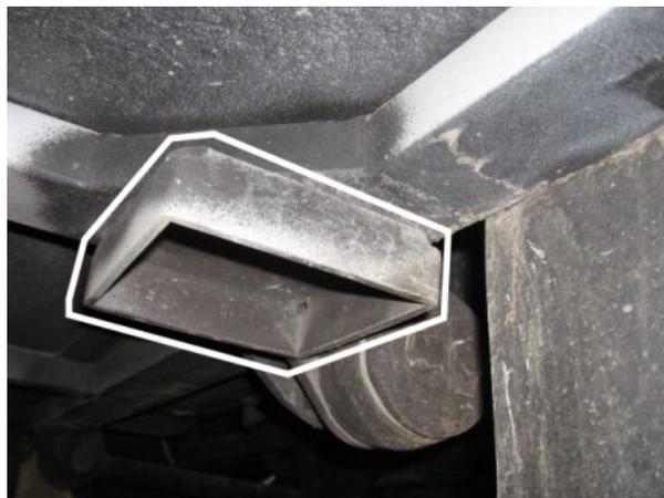
**FIGURE 16: SUPPORT DE LEVAGE AU CHÂSSIS
