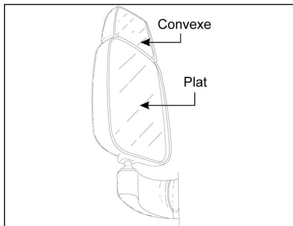
FIGURE 15 : RÉTROVISEUR (RAMCO)
