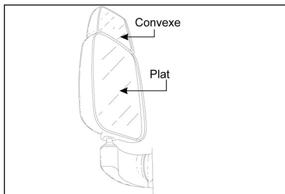
FIGURE 95 : RÉTROVISEUR (RAMCO)
