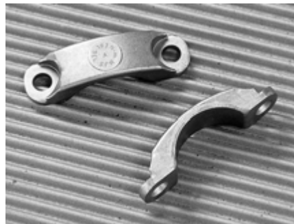
FIGURE 12: COLD FORMED BEARING RETAINERS
