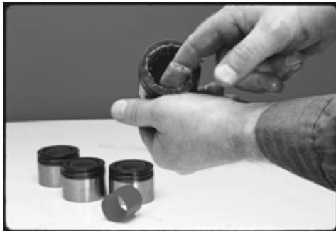
FIGURE 27: GREASING BEARING CUP
