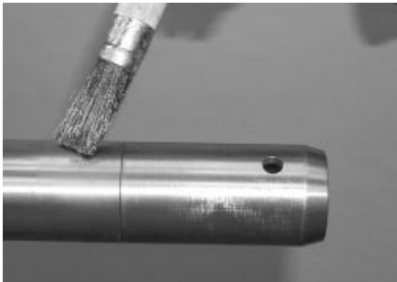
FIGURE 19: APPLY GLEITMO 805 GREASE
