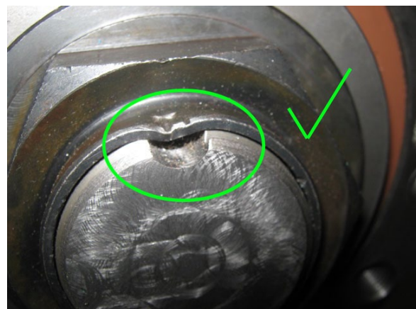
FIGURE 24: CORRECT - PREVENTS THE NUT FROM GETTING LOOSE
