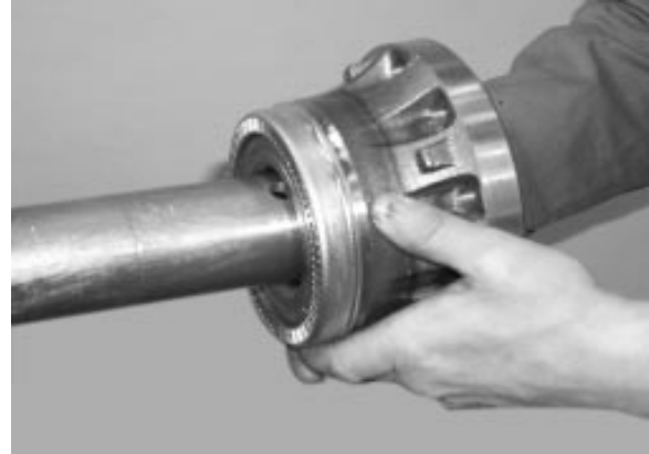
FIGURE 20: SLIP UNITIZED HUB BEARING OVER SPINDLE
