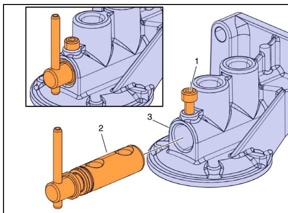
FIGURE 10: INSERTION DU CYLINDRE
