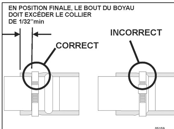
FIGURE 13: INSTALLATION CORRECTE DES COLLIERS DE SERRAGE
