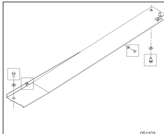
FIGURE 50: VIS DE MONTAGE DU PROTECTEUR ANTI-ÉCLABOUSSURE
