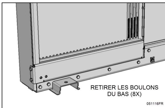
FIGURE 62: VIS DE LA SECTION AVANT INFÉRIEURE
