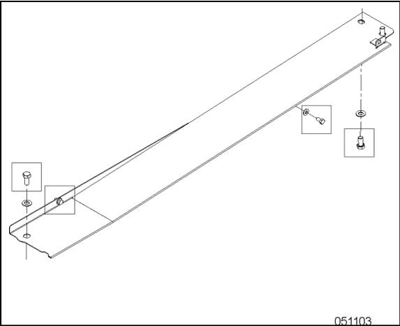
FIGURE 34: VIS DE MONTAGE DU PROTECTEUR ANTI-ÉCLABOUSSURE
