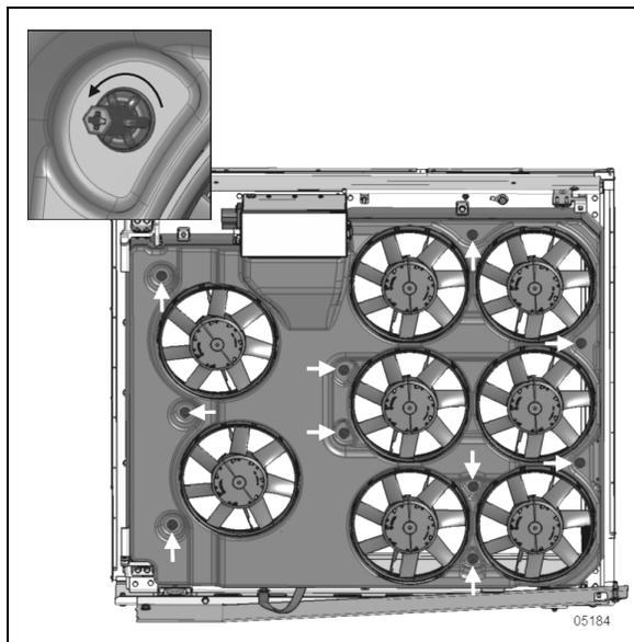
FIGURE 22: POSITION DES ATTACHES DU COUVERCLE DE PROTECTION
