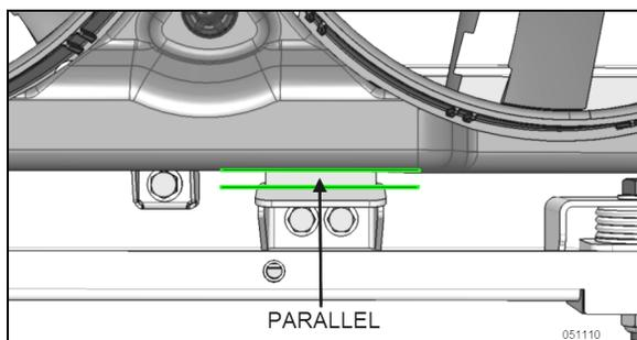
FIGURE 56: AJUSTEMENT DU BAS DU CARÉNAGE AVEC LE SUPPORT INFÉRIEUR
