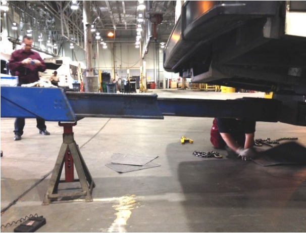
FIGURE 62 : PROPER LOCATION WHEN LIFTING THE SIDE MEMBERS – VEHICLE EQUIPPED WITH REAR TOW EYES
