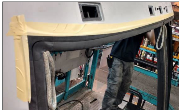
FIGURE 63: MASKING TAPE APPLICATION
