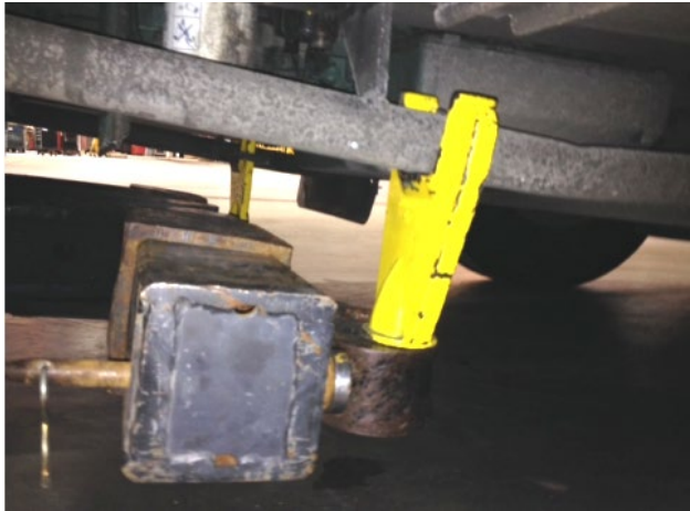
FIGURE 61 : PROPER LOCATION WHEN LIFTING THE SIDE MEMBERS
