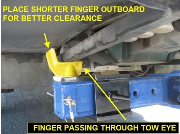
FIGURE 62 : PROPER LOCATION WHEN LIFTING THE SIDE MEMBERS – VEHICLE EQUIPPED WITH REAR TOW EYES
