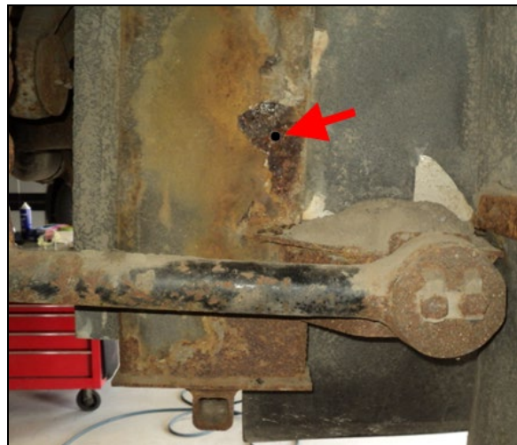
FIGURE 7: HOLE DRILLED IN STRUCTURAL MEMBER
