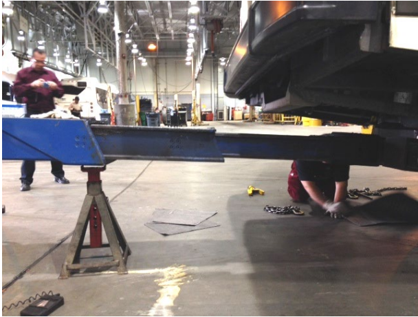
FIGURE 62 : PROPER LOCATION WHEN LIFTING THE SIDE MEMBERS – VEHICLE EQUIPPED WITH REAR TOW EYES
