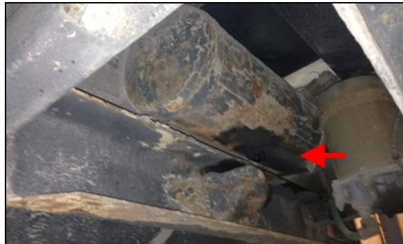
FIGURE 9: APPLICATION DE TECTYL 185GW BLACK
