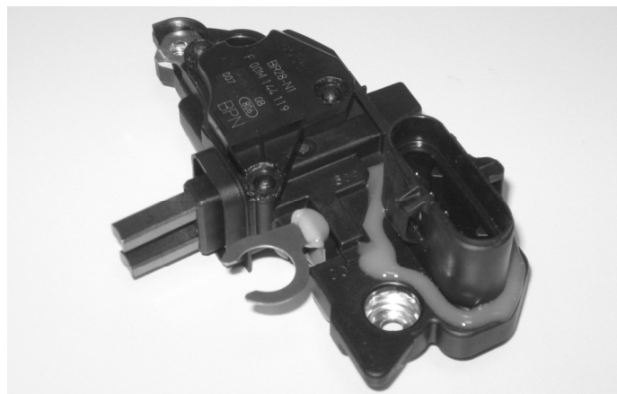
FIGURE 4: BRUSH HOLDER AND VOLTAGE REGULATOR ASSEMBLY
