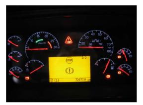
Confirm that rear circuit is at 0 PSI and that front circuit is 70 PSI. Pressure in the third axle tank should remain at 110 PSI. Warning telltale lights are ON and parking brake remain released.
