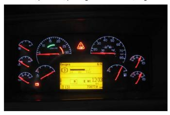
2. Use the cluster display to check third circuit air tank pressure. To do so, press "Enter", choose "Gauge mode", go to screen (3) that shows 3rd axle air pressure (See picture below)
