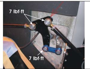
8. Reinstall wiper arms to their original position by aligning the marks made during removal. Do not forget to reinstall the O-ring (item #5).
