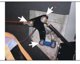
7. Inside the vehicle, fasten linkages to the pivots mounting plate (see picture at right).
