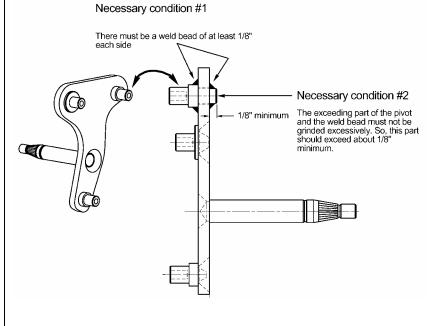
Part is not up to the standards of quality and must be replaced in the following cases (see figure at right).
