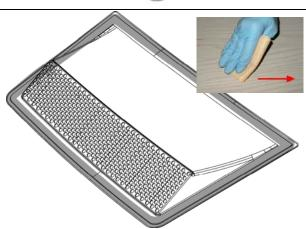
6. Apply 1/8X1/4 double-face adhesive tape around the air grille at about 1/8 inch from the edge.
