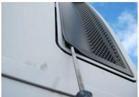
ON THE PICTURES ABOVE, INSERTING A SCREWDRIVER SHOWS WEAK BONDING (protect surrounding painted surface)
