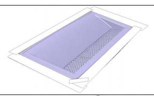
2. Using making tape, protect the painted surface of the air grille.
