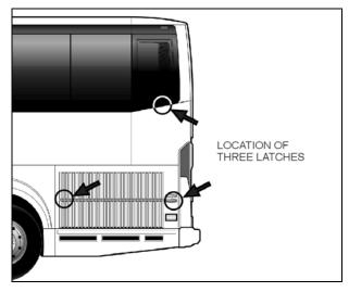
3. Check that there is a small play between the latch bolt and the faceplate. Validate that the latch bolt can move freely and that it returns to its normal position with the spring action when released. If the latch functions properly, no repair is required.
