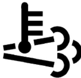
High Exhaust System Temperature (HEST)
