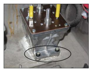
14. Tighten the three (3) hex nuts to 16 ft-lb (22 Nm).
