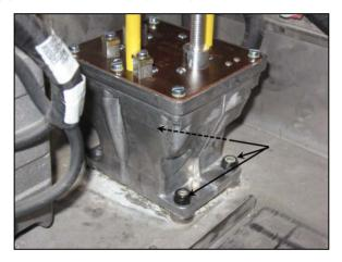
15. Reconnect the two (2) secondary wires at the top of the relay (flat head screws).
