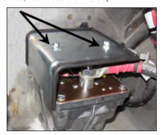
19. Re-install the rear right battery in the battery box (negative post goes left positive one right as shown below)
