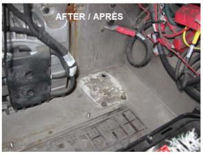
12. With the help of an assistant, install the three (3) new 30mm bolts from under the vehicle and slide the six (6) stainless flat washers over the bolts treads in the battery box.
