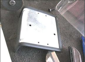
18. Using the two (2) hex nuts, install the cover on the relay.
