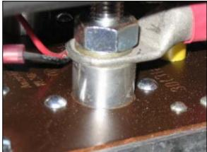
8. Disconnect both secondary connections (two (2) flat head screws).
