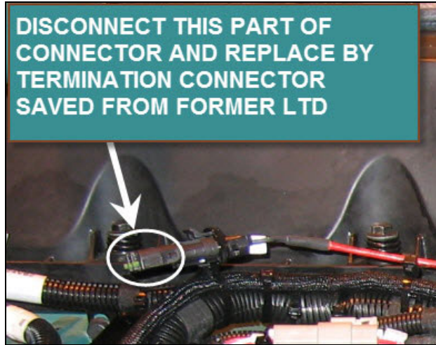
STEP 3 H: TERMINATION CONNECTOR
