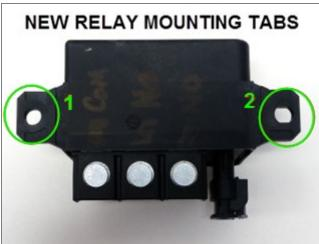
6. Trial fit the new relay into position, in most cases; the new relay will have to be mounted at an angle to clear the connectors and surrounding relays as shown in the figure below.
