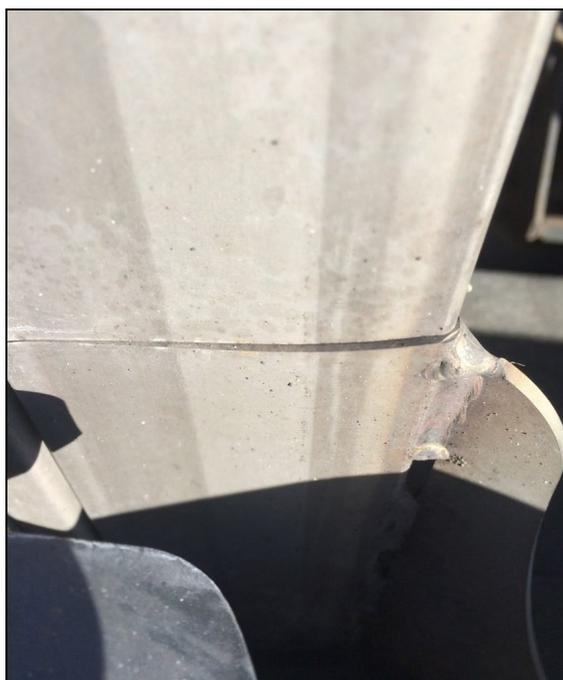
On these vehicles, it is possible to install and weld a frame reinforcement in the rear frame support beam to repair the affected area.
