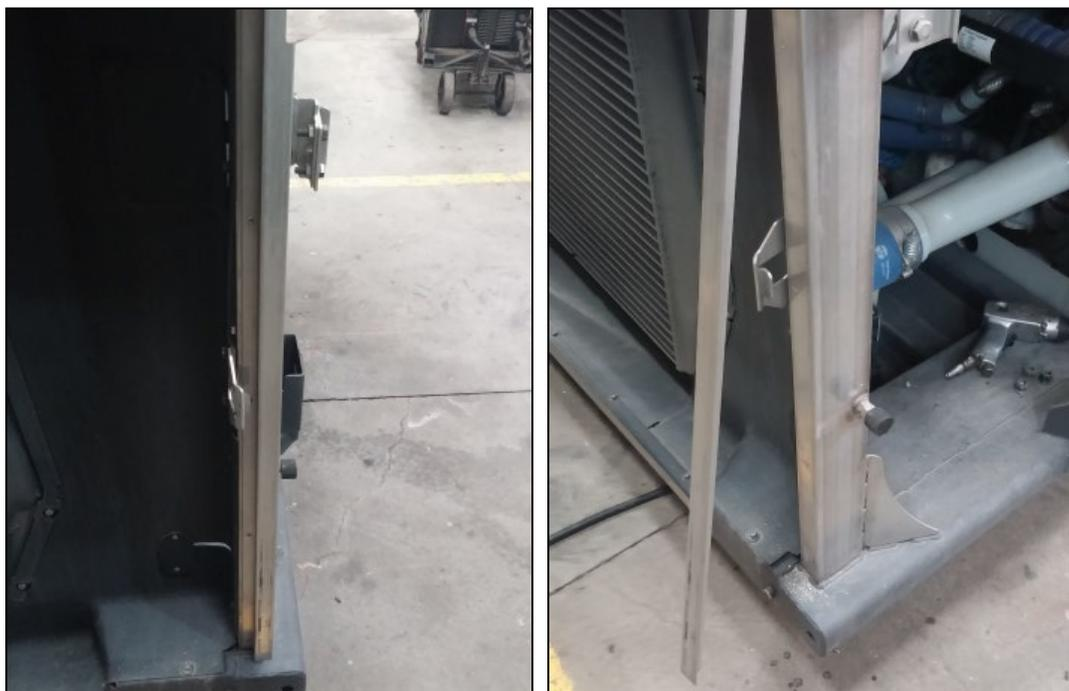
4. Remove the rearmost plastic radiator shroud and metal hold down support using a 10mm socket (15 hex bolts).
