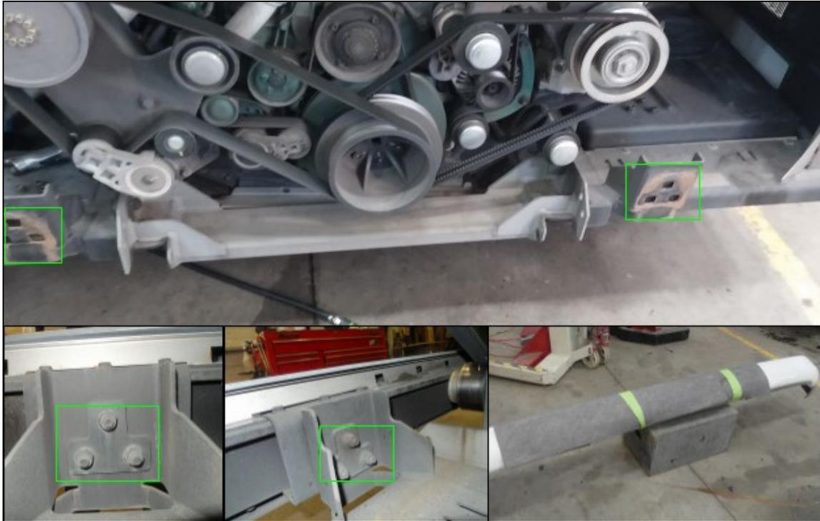
3. Open the left engine door and remove the stainless steel trim riveted to the left rear support beam (use an electric drill and suitable drill bit to remove the rivets).
