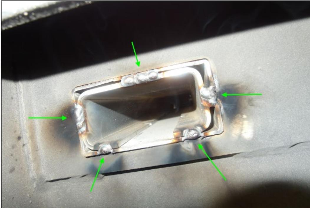
11. Weld the entire length of the enlarged crack ensuring of proper weld penetration trough the support reinforcement.
