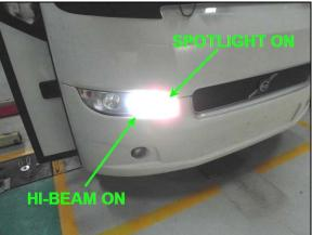
If the spot lights fail to light or they only blink on and go off, the vehicle Lighting Control Module (LCM) harness pin out must be modified as per the drawing below.
