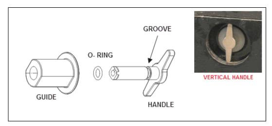
14. Position the latch plate square opening over the handle tip (make sure again that the handle is vertical).
