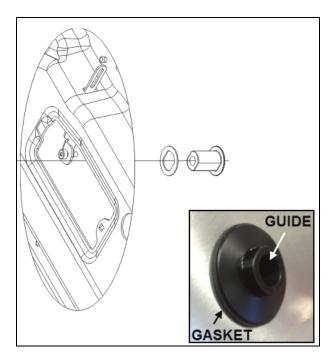
12. Install another guide gasket (280477) inside the door opening and secure the handle guide to the door using the provided flat washer (5000350) and M20 lock nut (5000351).
