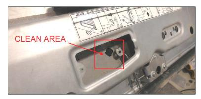
7. Insert black plastic handle guide (280474) (cylinder lock replacement) into the door opening (from the outside) making sure that the guide flat sides are installed left & right as shown.
