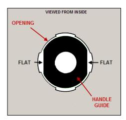
8. Peel the protective paper off the support plate (280781) two sided tape strips and slide the plate over the handle guide (from inside door opening). Make sure the plate and the guide flat side are installed as shown below and press slightly to ensure complete adhesion of the plate to the door.
