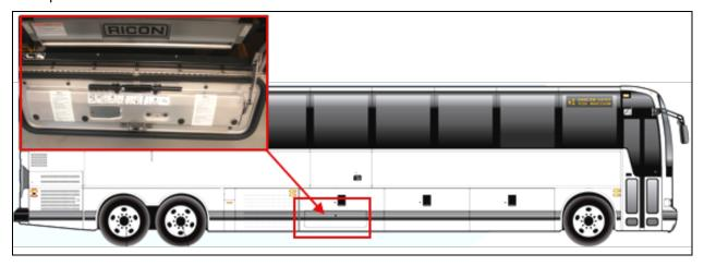
2. Remove the lock mechanism back cover (Phillips head screw and plastic washer).
