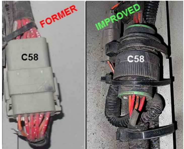
Figure 18 : C58 ARRANGEMENT "FORMER" AND "IMPROVED"
