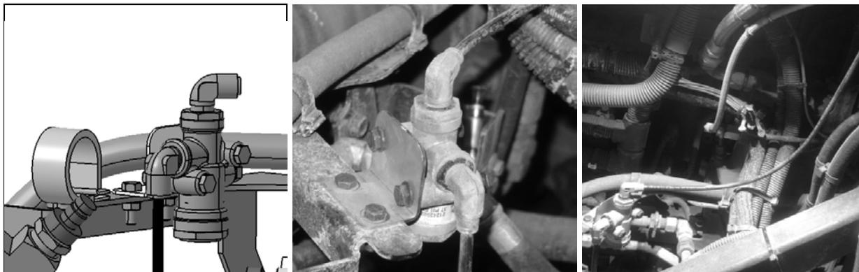
RV-3 VALVE INSTALLED – NEW LOCATION
