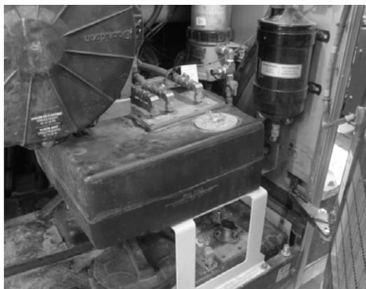
3. Inspect the valve (and air connection) to make sure that it is in good condition and not leaking. Order a new valve as required (part # **21243502**).
