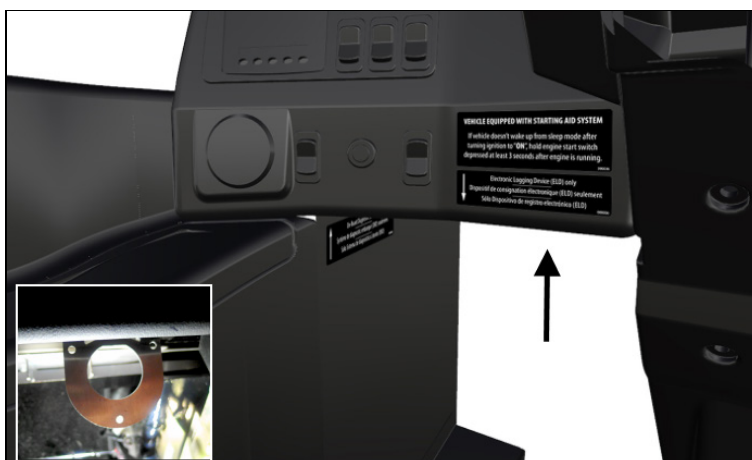
BRACKET POSITION UNDER DASH
