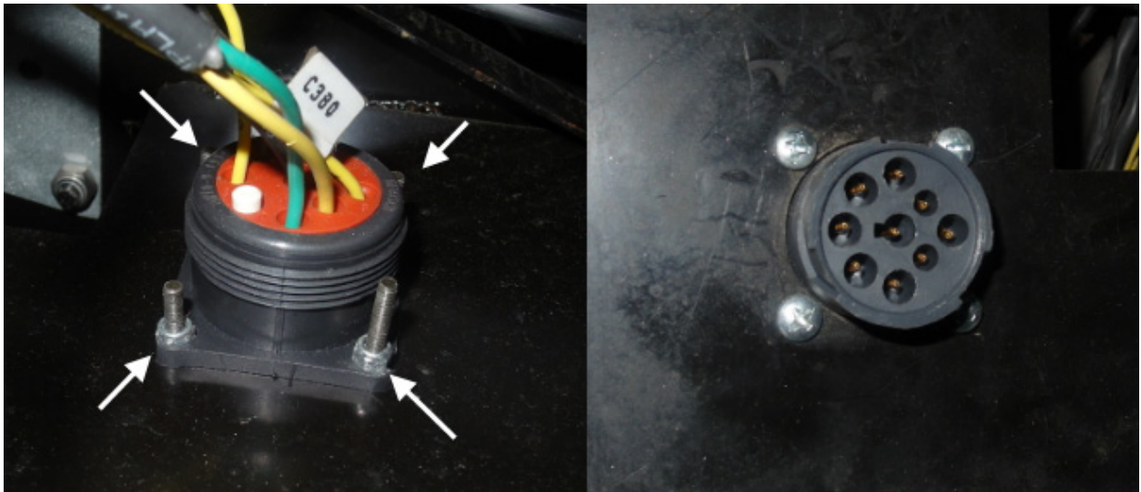
DIAGNOSTIC CONNECTOR SCREWS; BOTH SIDES
