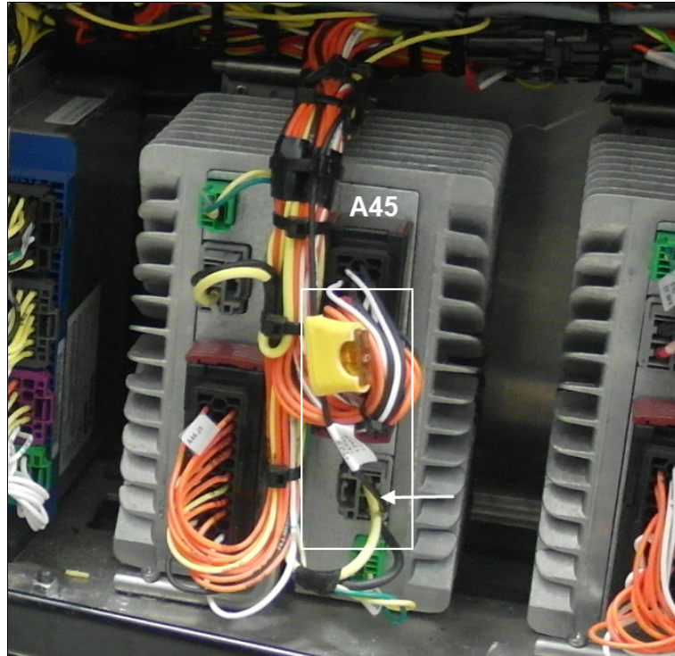
A45 MODULE & ELD GATEWAY MODULE CONNECTION
