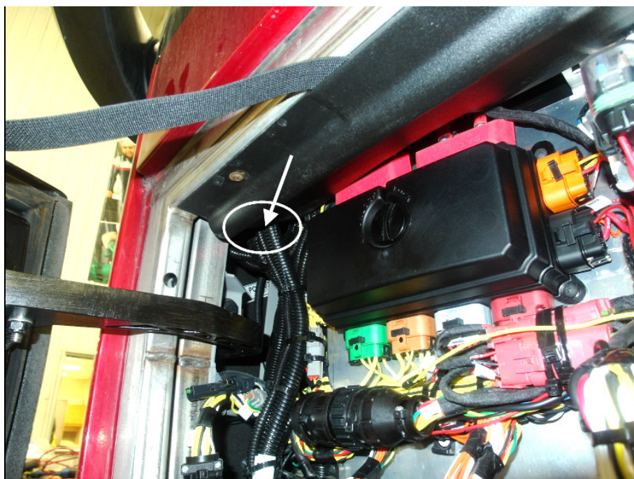
AVOID CONTACT HERE ON H3 VEHICLES
