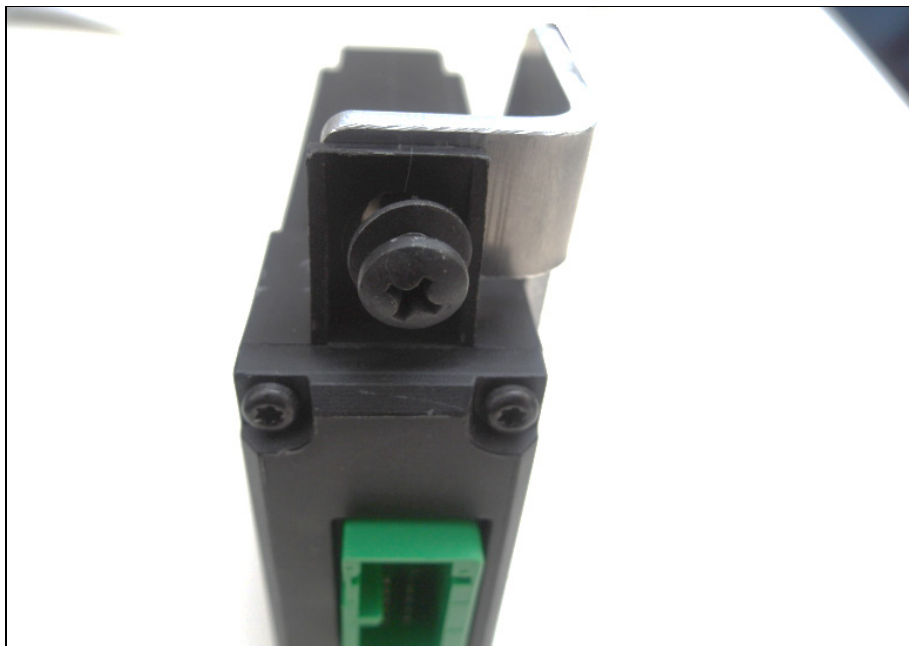
GATEWAY MODULE ON BRACKET – USE FLAT WASHERS
