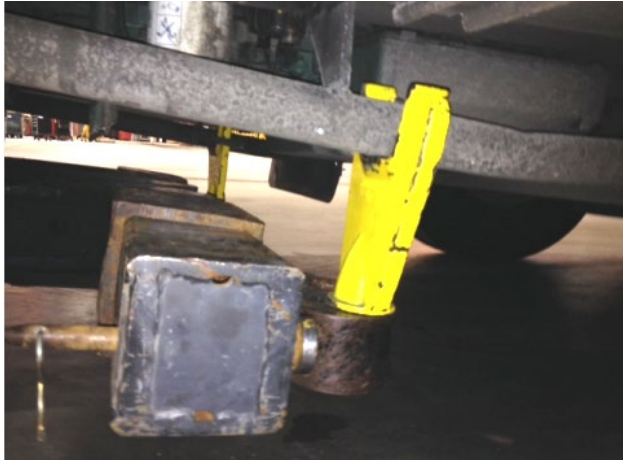
FIGURE 61 : PROPER LOCATION WHEN LIFTING THE SIDE MEMBERS
