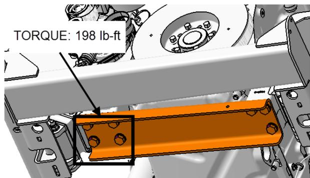
**FIGURE 38: FOUR (4) SCREWS UNDER THE REINFORCEMENT CHANNEL**
