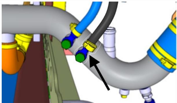
FIGURE 74: DEF INJECTOR COOLANT LINE RETURN HOSE
