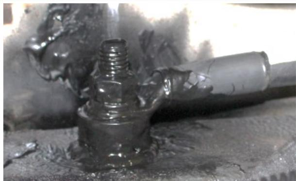
FIGURE 83: GROUND STUD WITH RUBBER COATING
