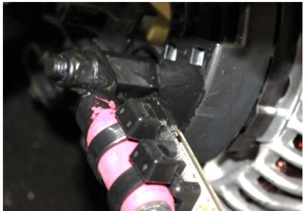
**FIGURE 85: POSITIVE (+) CONNECTION ON THE ALTERNATOR**
