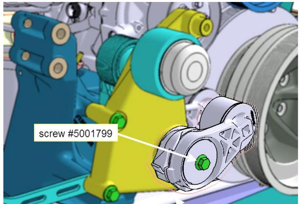
FIGURE 49: TENSIONER MOUNTING SCREW TORQUE : 48 lb-ft
