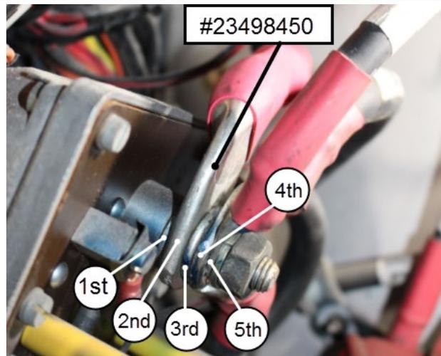
FIGURE 155: ON THIS PICTURE, CABLE #23498450 LUG IS IN SECOND (2<sup>ND</sup>) POSITION BECAUSE IT WAS LIKELY TO RUB ON THE HEAD OF ONE OF THE FOUR SCREWS.
