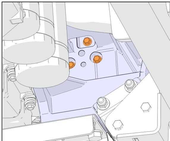
FIGURE 49: IDLER / TENSIONER ASSEMBLY MOUNTING SCREWS
