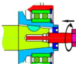
PULL OFF THE ROTOR WITH TOOL #680888 (shown)
