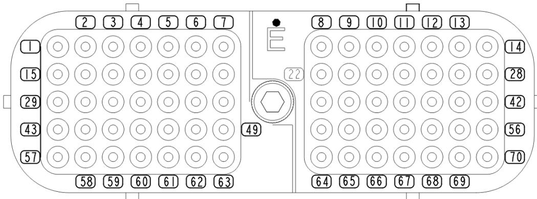
FIGURE 6: C397 PINOUT
