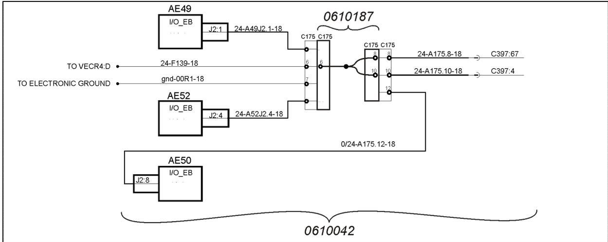
FIGURE 3: 0610042 & 0610187 HARNESS CONNECTIONS IN MAIN POWER COMPARTMENT
