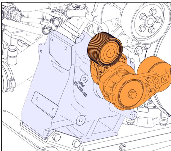
FIGURE 48: KEEP IDLER/TENSIONER ASSEMBLY INTACT
