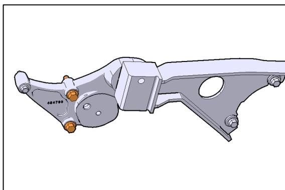
FIGURE 14: VARIANTE AVC RENFORT SOUDÉ (2013-2015)
