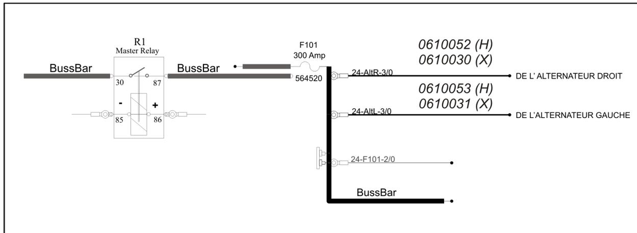
**FIGURE 2: CONNEXIONS DES CÂBLES D'ALIMENTATION DANS LE COMPARTIMENT D'ALIMENTATION PRINCIPAL**
