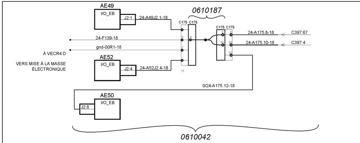
FIGURE 3: CÂBLAGE 0610042 ET CAVALIER 0610187 DANS LE COMPARTIMENT D'ALIMENTATION PRINCIPAL.
