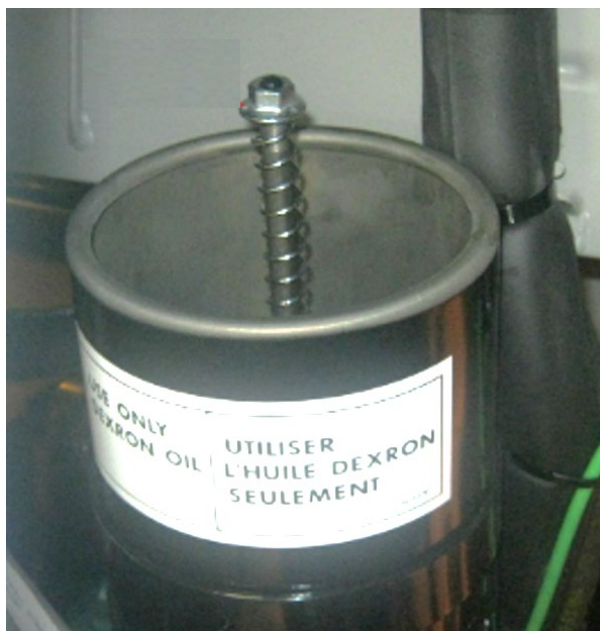
FIGURE 26: POWER STEERING FLUID TANK
