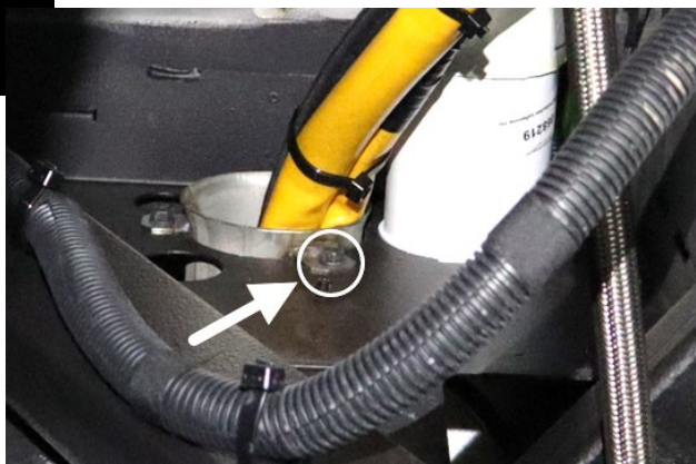
FIGURE 44 : FLARED STEEL TUBE
