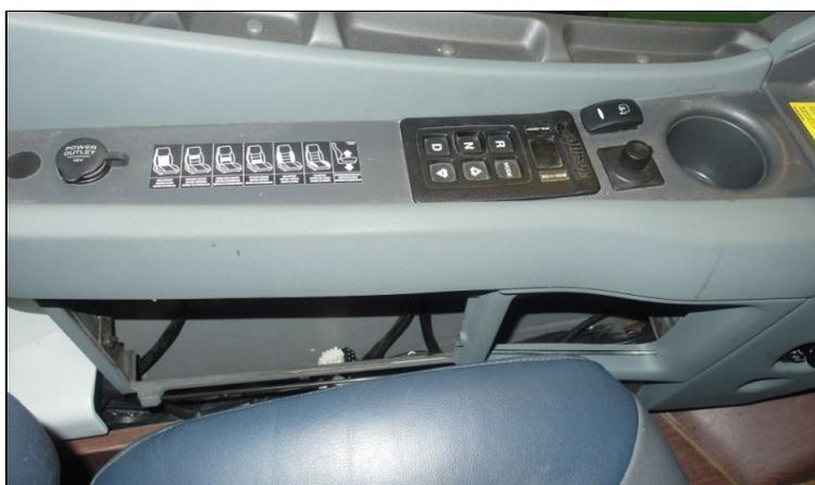
3. Route the ELD interface harness **23446645** from the electrical compartment up to the driver's area (diagnostic connector area).
