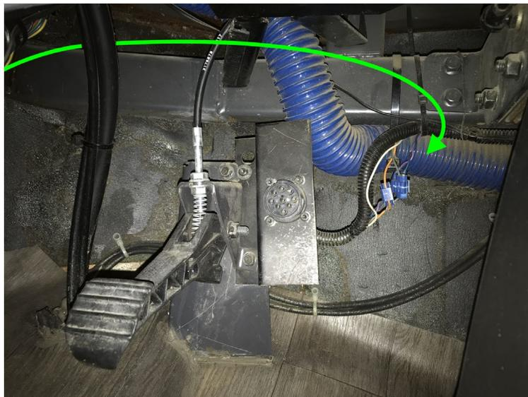
4. Remove the vehicle 9 PIN diagnostic connector from the underside of the dashboard (drivers' side).
