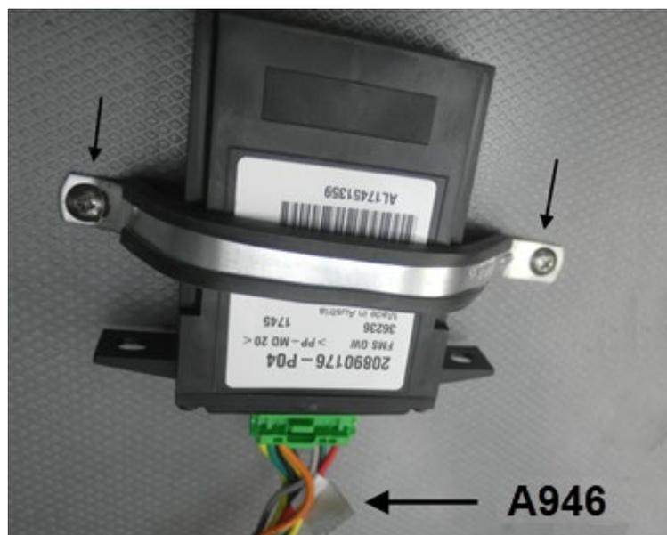
8. (Optional step) If using a Volvo branded ELD device (part # 7770385). Secure the ELD device next to the gateway module using the supplied #24 Adel clamp **952634** (connector facing down).
