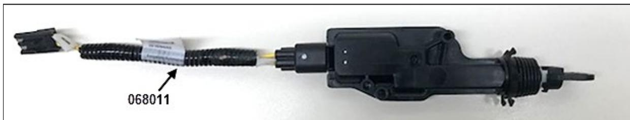
6. Secure the new **2800049** actuator to the **2810380** adaptor bracket (Use supplied **5001100** screws, **500437** washers & **5001408** nuts). The tip of the actuator must be mounted toward the “straight” (90deg angle) part of the adaptor.
