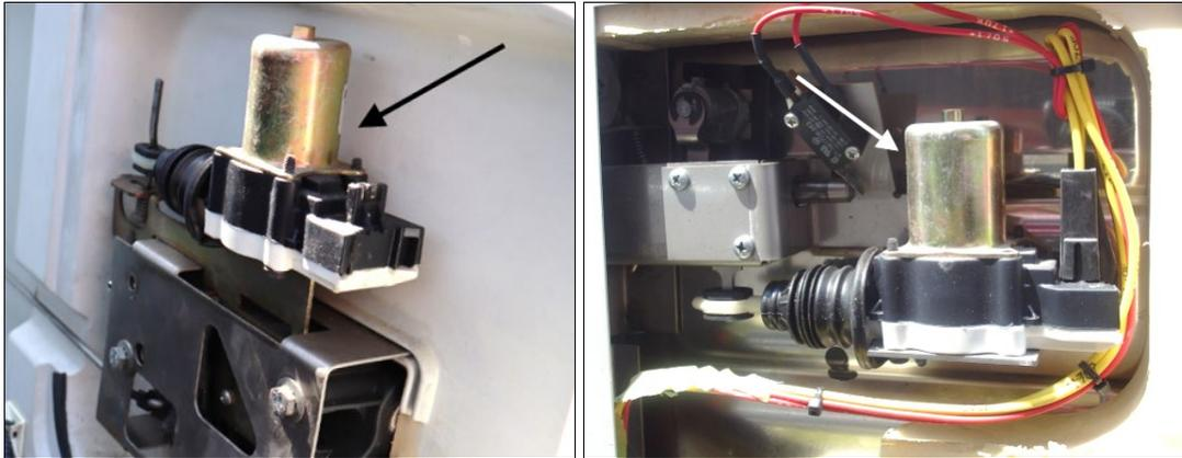
2. Snugly install the **2810380** adaptor bracket to the original actuator support using only the front bolt (use supplied M4 screw, washer & nut). *The adaptor must fit squarely with the support.*
