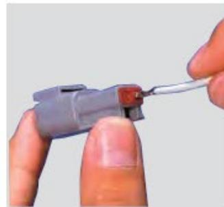
3. Push contact straight into connector grommet until a click is felt. A slight tug will confirm that it is properly locked in place.
