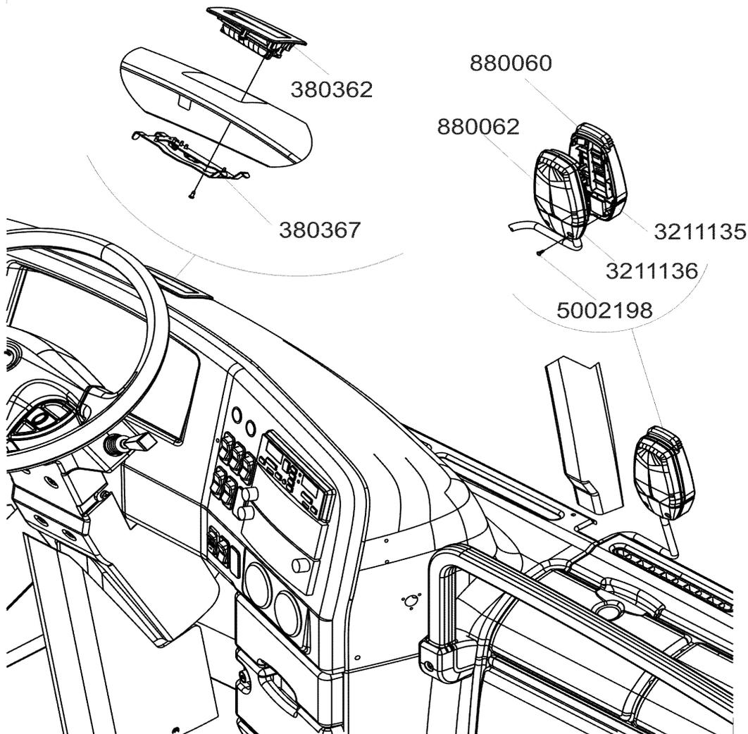
FIGURE 1: WINDSHIELD CAMERA (RIGHT) & HEAD-UP DISPLAY (LEFT)
