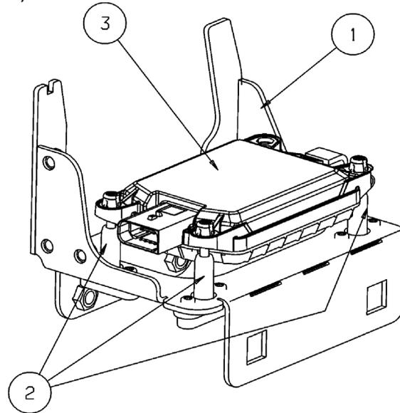
**STAND-OFF ADJUSTERS ARE NOT REUSABLE. DO NOT SEPARATE THE RADAR SENSOR FROM THE STAND-OFF ADJUSTERS IN ORDER TO REPLACE A DEFECTIVE RADAR SENSOR.**
