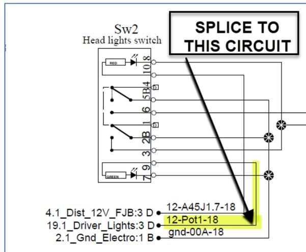
FIGURE 38: SWITCH SW2 HEADLIGHTS
