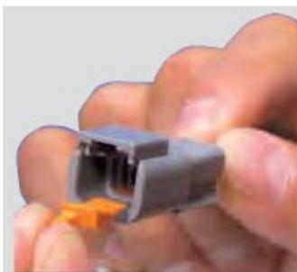
4. Once all contacts are in place, insert orange wedge: receptacles - with half holes aligning with contacts. Plugs - with contacts aligning behind full holes. The orange wedge will snap into place.
