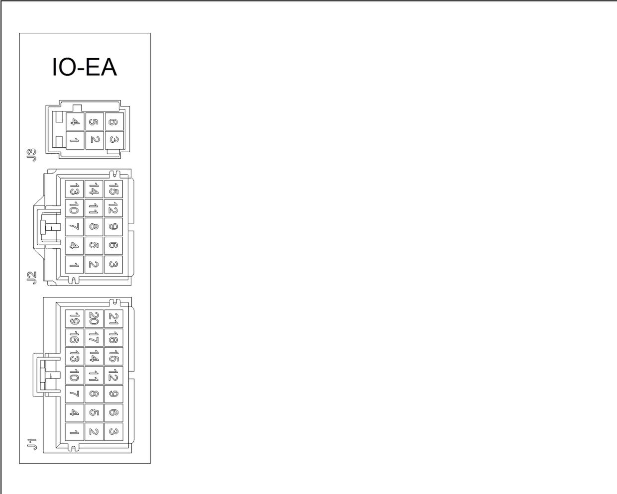
FIGURE 86: ELECTRONIC MODULE CONNECTOR PIN-OUT - BACK PROBING VIEW
