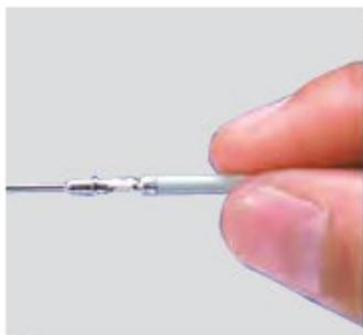
1. Grasp crimped contact approximately 1.0" (25.4mm) behind the contact barrel.
