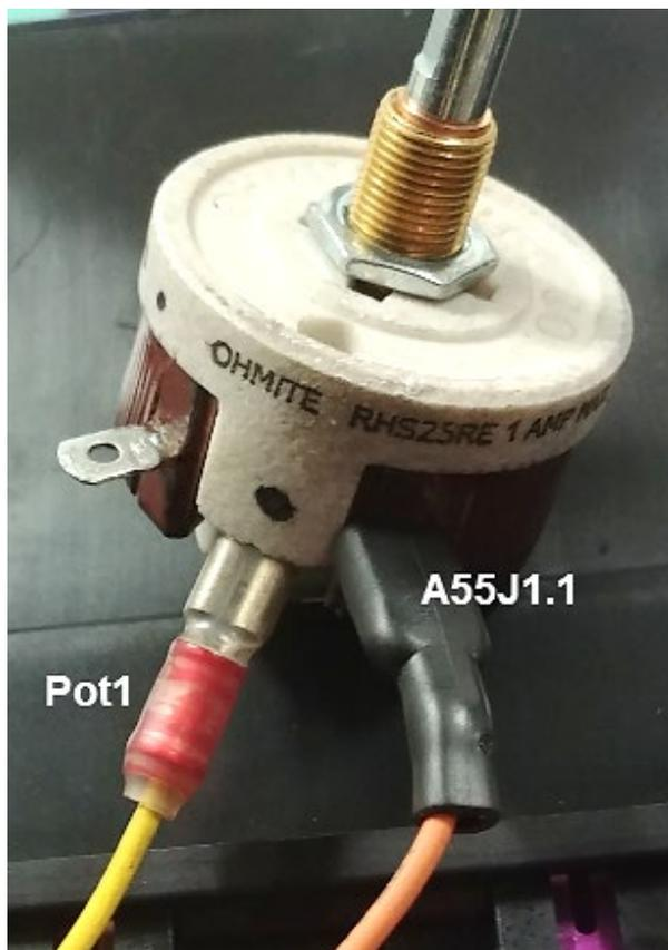
8. Install the potentiometer on the vehicle dashboard.
