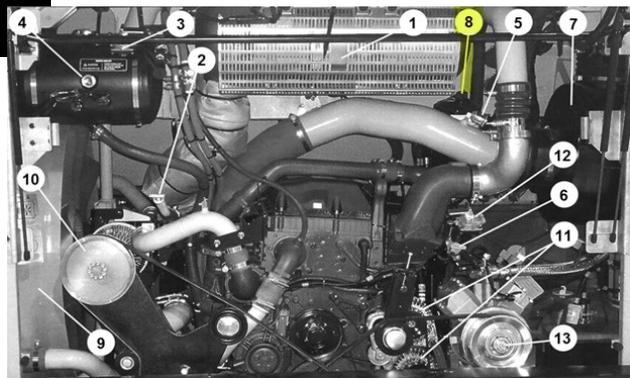
FIGURE 26: POWER STEERING FLUID TANK, ITEM 8 ON PICTURE ABOVE
