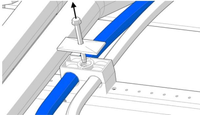
**FIGURE 7 : SPLIT BLOCK #1 IN THE SPARE WHEEL COMPARTMENT**
