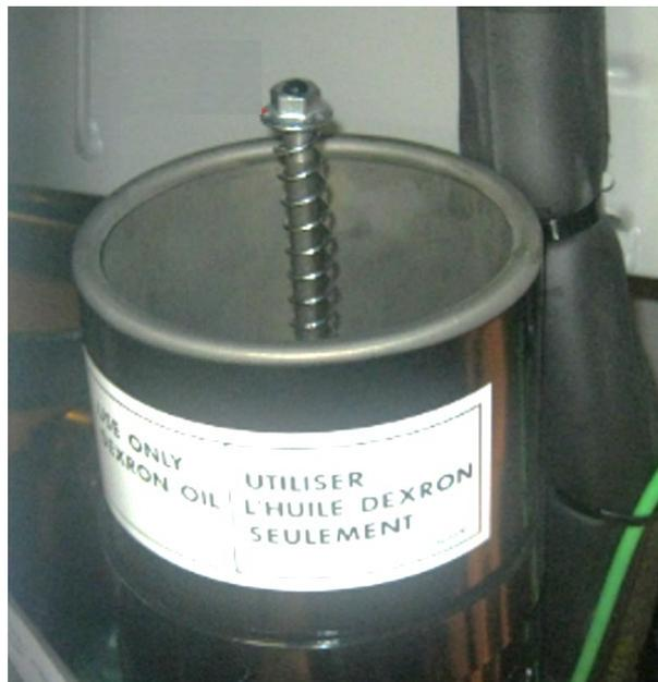
FIGURE 27: POWER STEERING FLUID TANK
