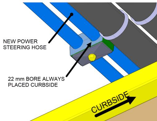
FIGURE 24: SPLIT BLOCK -TYPICAL INSTALLATION
