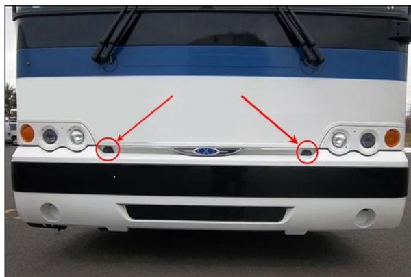
FIGURE 29: BUMPER TOP RETAINING BOLTS
