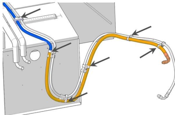
FIGURE 6 : TWO (2) P-CLAMPS, THREE (3) HOSE GUIDES, ONE (1) SPLIT BLOCK
