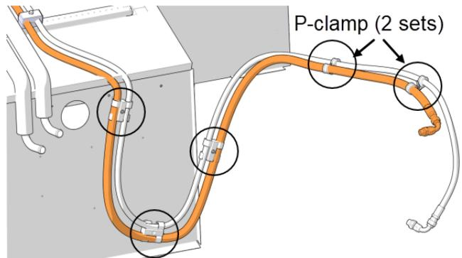
FIGURE 25 : TWO (2) P-CLAMPS, THREE (3) HOSE GUIDES
