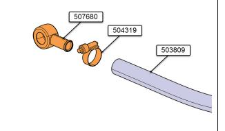
B) With Detroit engine assemble Hose 503809 and fitting 7772004 and collar 504319.
