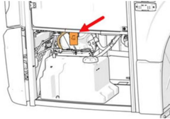
2. Pull out the safety catch on the inside top right-hand side of the hatch.
